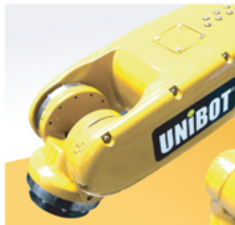
Electrical and pneumatic near tool flange.
